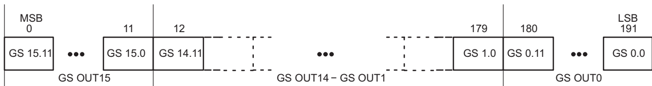
Figure 17. Grayscale Data Packet Format
