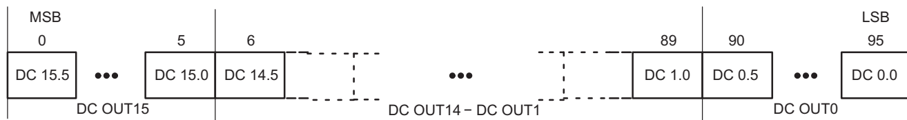
Figure 15. Dot Correction Data Packet Format
